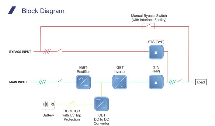
"Monolithic" – it used to describe a system that is made up of single sub-systems (Rectifier, Battery charger, Inverter, Bi-Directional static switch etc.) with no intrinsic multiple modules. Monolithic UPS have less number of components, which increases the reliability and reduce the mean time between failures (MTBF) that ultimately beneficial to user.
