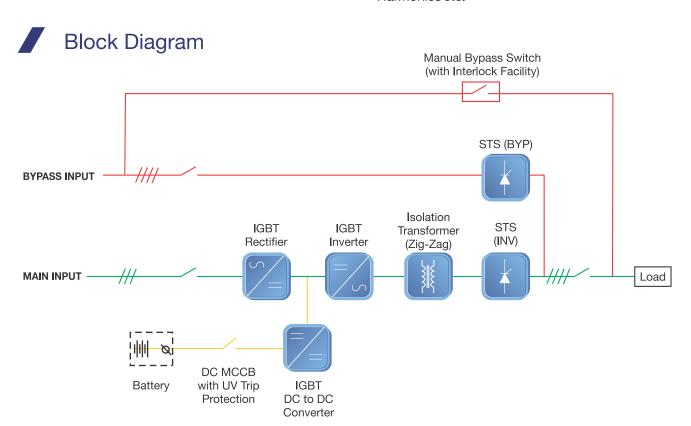
"Monolithic" – it used to describe a system that is made up of single sub-systems (Rectifier, Battery charger, Inverter, Isolation transformer, Bi-Directional static switch etc.) with no intrinsic multiple modules. Monolithic UPS have less number of components, which increases the reliability and reduce the mean time between failures (MTBF) that ultimately beneficial to user.
